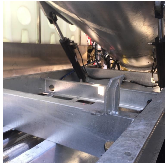
Hydraulic Rams used to lift and tilt tank to empty contents. Pressure protection valvue and Anti Drop Value installed to prevent uncontrolled movement in the event of a Hydraulic failure
