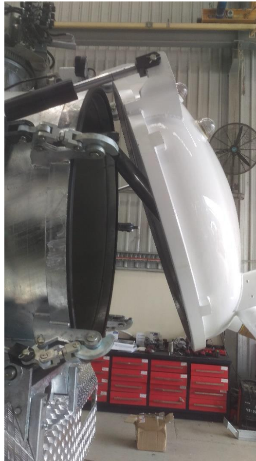
Door opening using hydraulic rams
