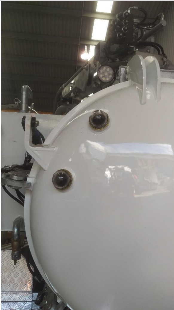
Inspection of the tank capacity during operation can be viewed through the glass elements on the door
