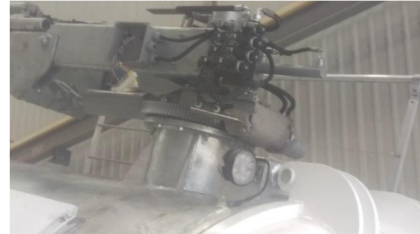
Exposed components at the rear of the plant connecting the boom to the tank. Shows exposed components. Therefore, isolation of the plant and equipment prior to climbing onto upper platform must occur and operators to be trained prior to use
