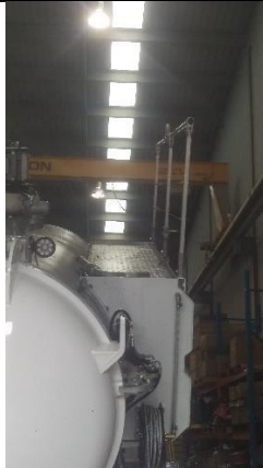
Handrail on upper platform erected to protect operator
