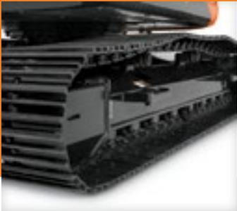
■ With large idlers, rollers, and struted links, the sealed and lubricated undercarriage delivers long, reliable performance.
