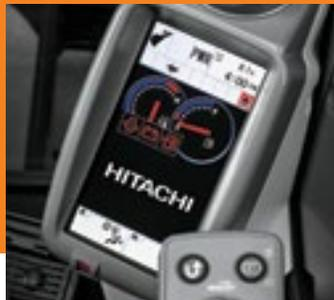
■ Multi-language LCD monitor and rotary dial provide access to a wealth of info and functions. Just dial and tap to check diagnostic codes, monitor maintenance intervals, set cab temperature and more.
