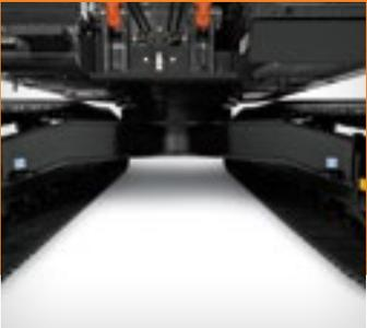
■ Box-section track frames, thick-plate single-sheet mainframe, and superior ground clearance and industry-exclusive double-seal swing bearing deliver rock-solid durability.
