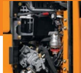
■ Vertical spin-on fuel filters are positioned in the right rear compartment for simplified ground-level servicing.
