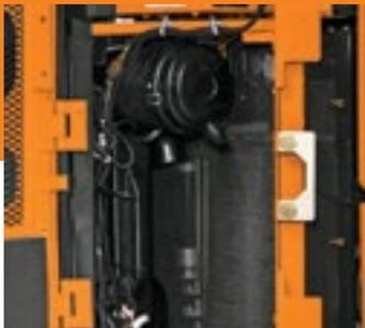
■ Left rear compartment houses the battery, engine air filter, fresh-air cab filter and side-by-side coolers.
